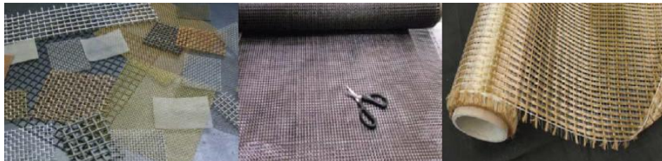
Figure 30- Fabric sheets of TRM made of steel, carbon, and PBO (Mininno, 2016)
