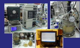
Fig. 2. Expression of recombinant bacteria was performed in a fermenter allowing large yields of rhBMP-2, around 110mg/L.
