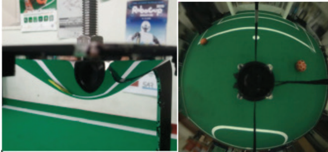
Figure 1 - Catadioptric Mirror and image captured by the catadioptric sensor
