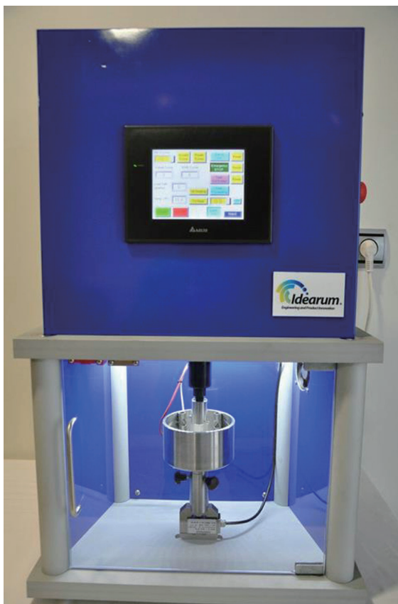
Fig. 1. CS- Dental Testing Machine® used in fatigue tests.
