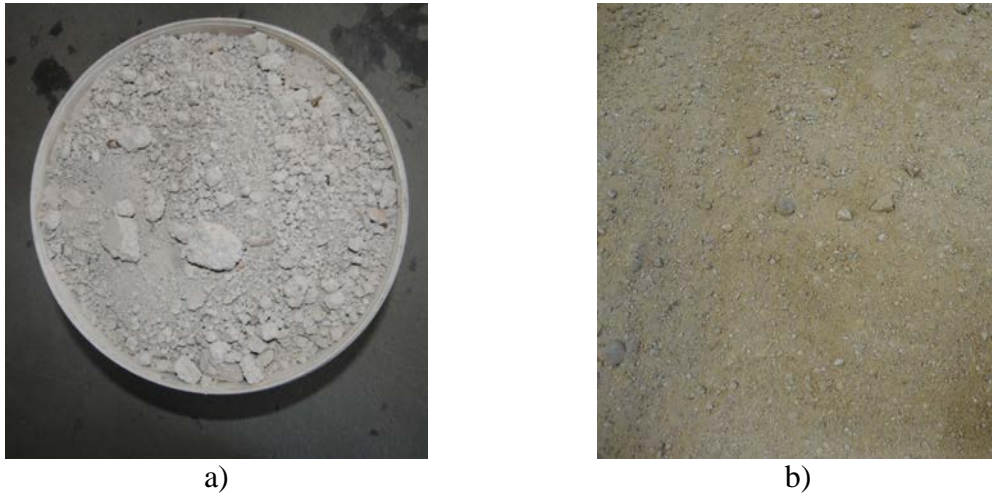
Figure 3: Studied materials in terms of granulometry: a) earth render of the reference tabique wall sample and b) collected soil
