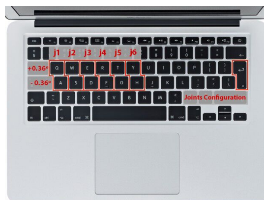
Figure 41 - Keyboard control implemented to input a precise configuration of each joint of the robotic arm.
