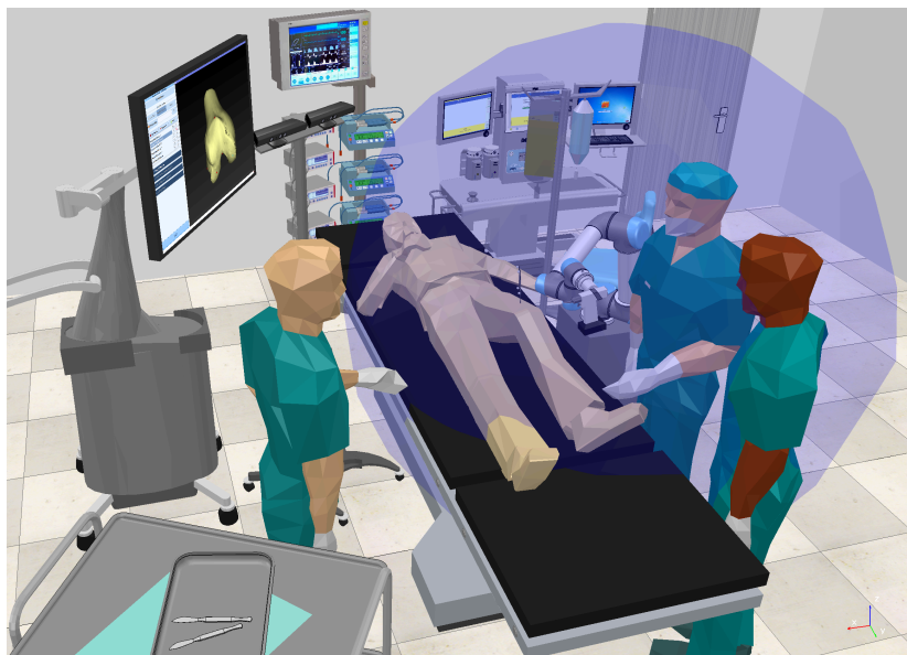
Figure 39 - Representation of workspace of robotic arm with the surgical instrument mounted.
