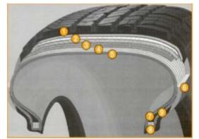
Fig. 1. Tire Structure [3]. Legend: 1 - Tire tread, 2 - Spiral textile band, 3 - Metal strip, 4 - Textile tire, 5 - Watertight layer, 6 - Tire wall, 7 - Tire bead wedge, 8 - Tire bead core, 9 - Tire bead reinforcement.
