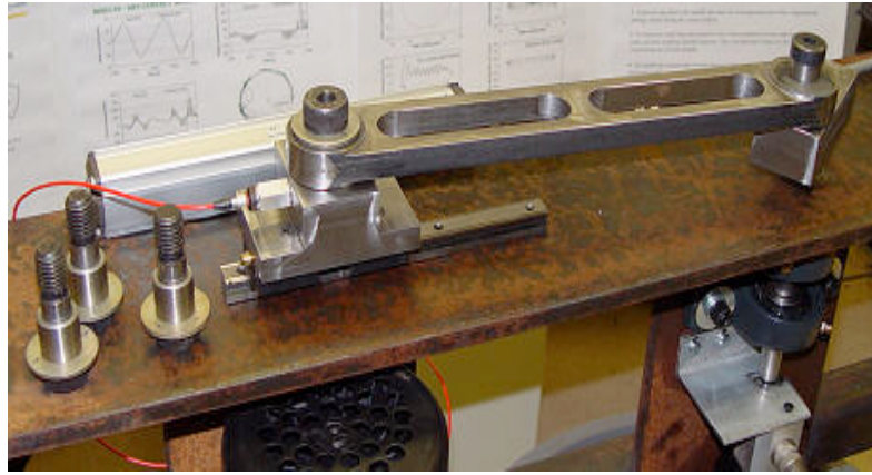
Fig. 40 Experimental slider-crank mechanism utilized by Koshy et al. [418].
