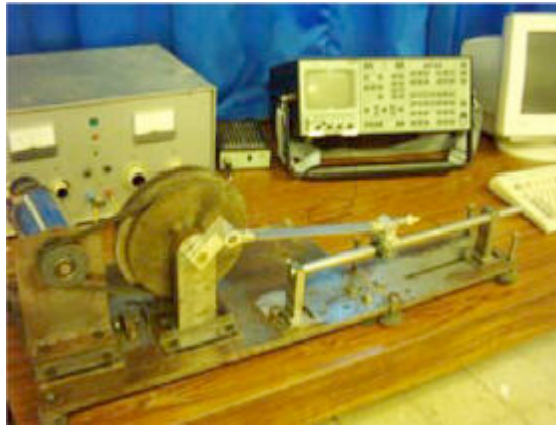
Fig. 35 Slider–crank mechanism with a flexible connecting rod [410].
