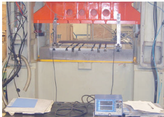
Fig. 38 The test platform of multi-link mechanism for high-speed press system [280].
