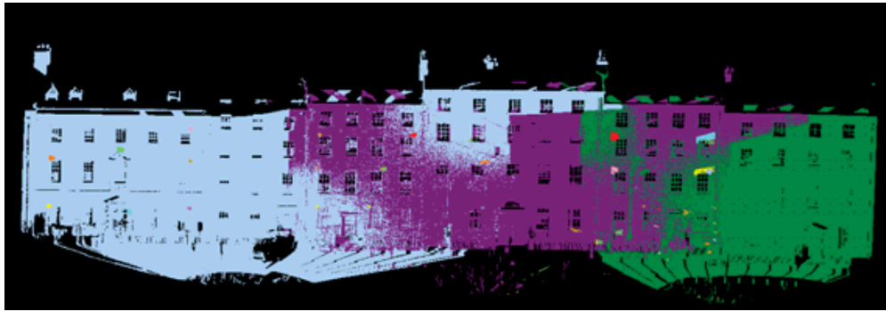
Figure 19 - Registration of first three scans (Dore and Murphy, 2012).
