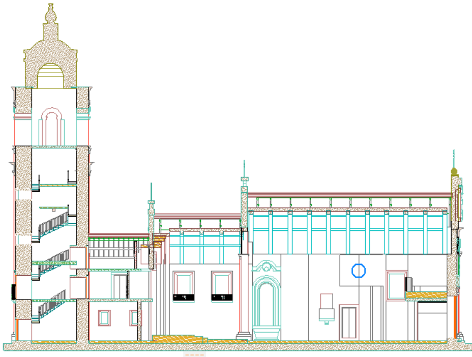
Figure 70 – Section along the centre of the church.
