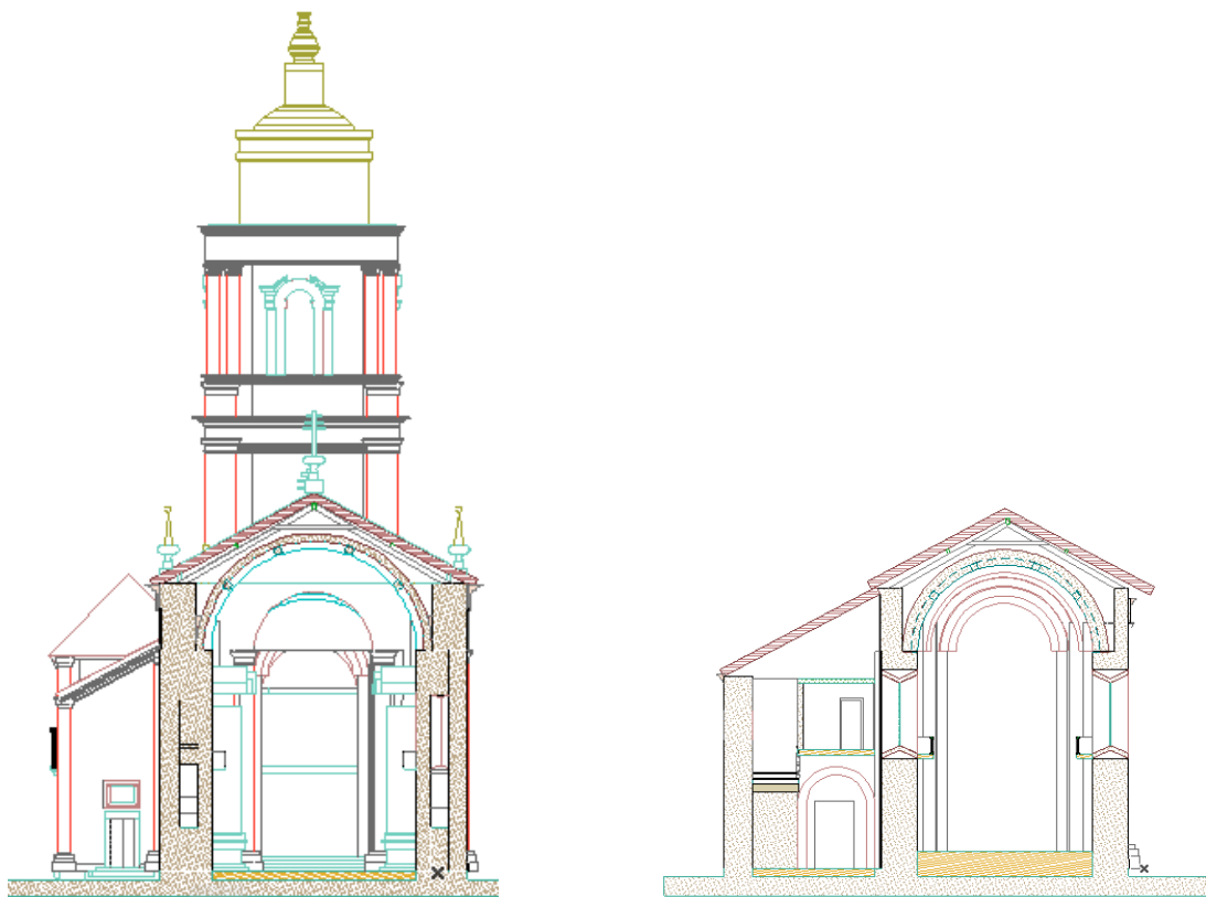
Figure 71 - Sections derived from the 3D BIM model.
