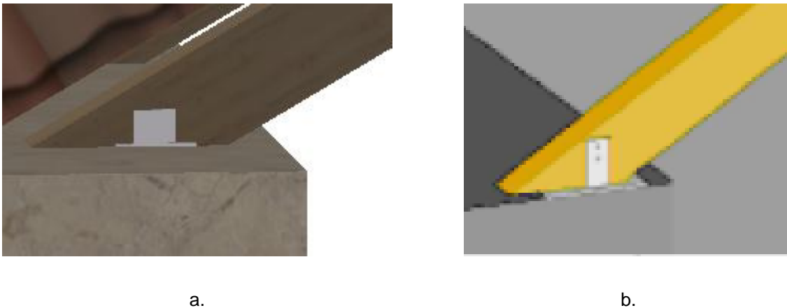
Figure 79 – a. Intervention on the roof derived from the 3D BIM model b. Intervention proposed (Betzer et al., 2014).
