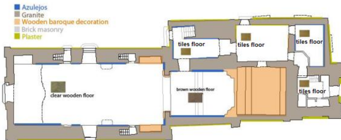
Figure 45 - Different materials present in the structure (Betzer et al., 2014).
