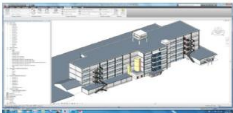
Figure 24 - Final HBIM model of the factory (Fai et al., 2011).
