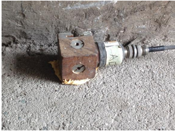
Figure 63 – Piezoelectric accelerometer attached to the structure
