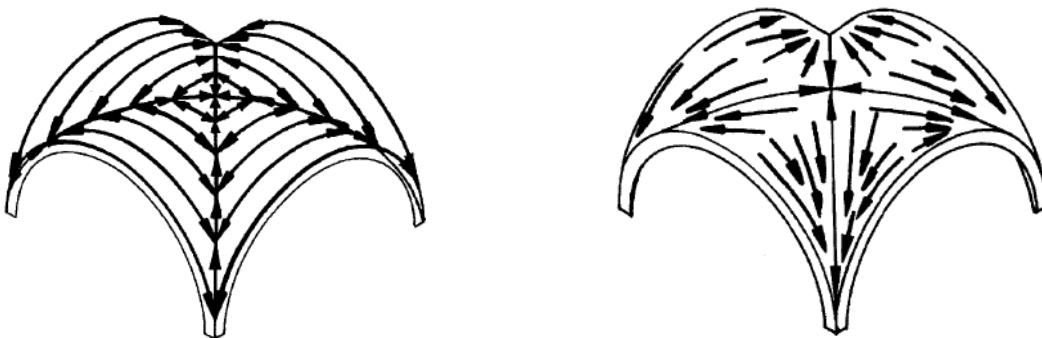
Figure 12 – Distribution of loads in groin vaults (O'Dwyer, 1999)
