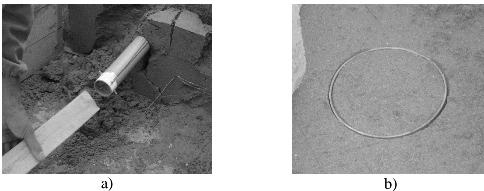
Figure 4.22. PVC tube introduction on the layer: a) laterally for EMM-ARM sample collection; b) from top for UCC testing
