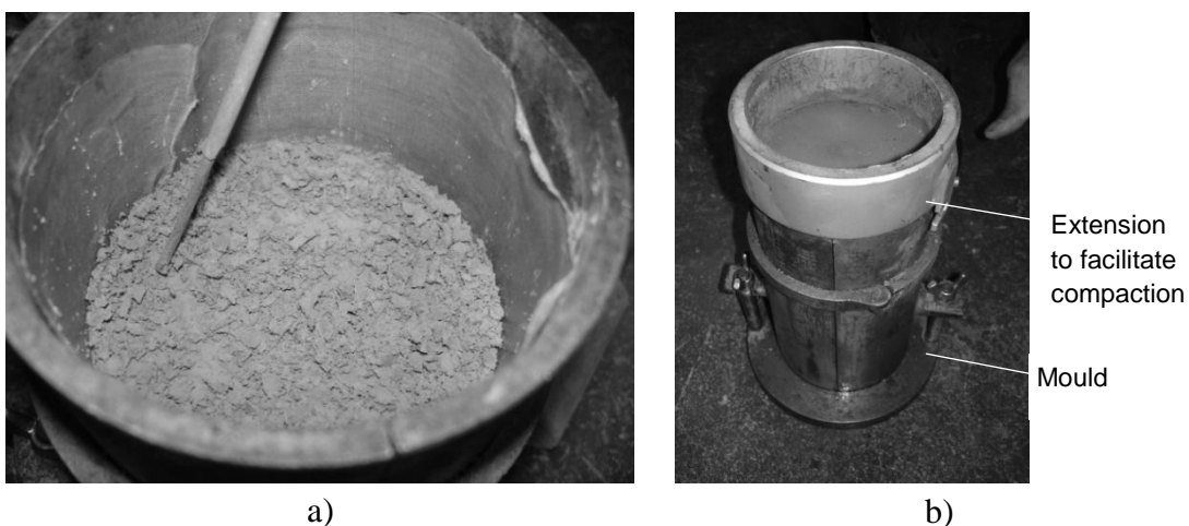
Figure 4.4. UCC specimen preparation: a) scarifying the surface of the layer; b) UCC specimen inside the mould with extension after final compaction
