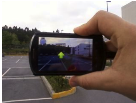
Figure 3: Augmented reality interface of the CogHelper Mobile Application for users with cognitive disabilities.
