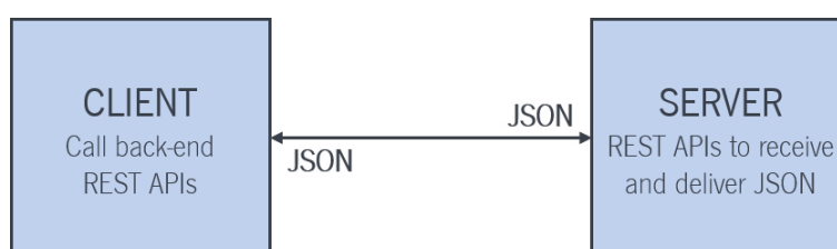
Figure 5.1: The REST architecture.
