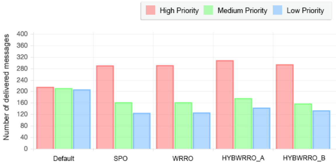
Figure 43.: Results for P Ro PHET Routing: Increased number of messages
