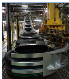
Figura 18-Green Tyres Conveyors (GTC)
