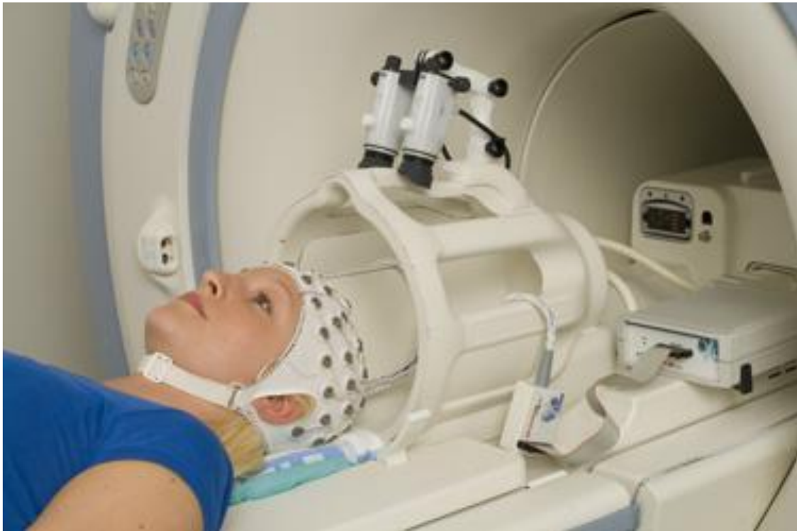
Figure 25: EEG-fMRI recording hardware setup [263].
