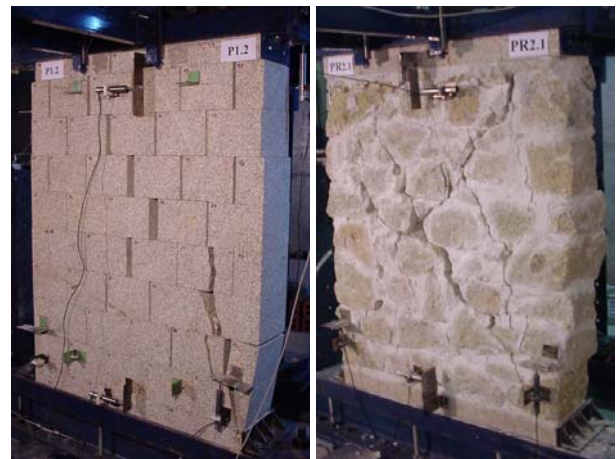
Fig. 3. Aspects of shear wall failure under cyclic loading, for regular and irregular stone masonry [6].
