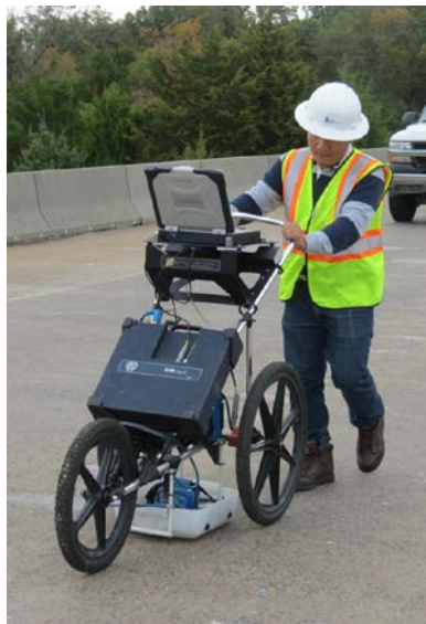
Fig. 4. GPR survey using a 1.5 GHz ground coupled antenna.
