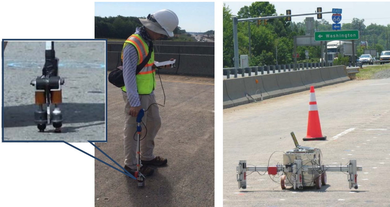
Fig. 6. Two types of IE testing systems: (a) an IE cane and (b) a stepper.
