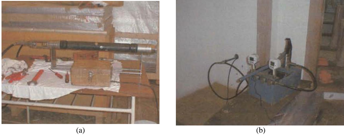
Figure 2-26 Dilatometer testing: (a) dilatometer; and (b) dilatometer inserted in drilled hole and oil pump for applying pressure
