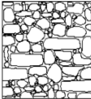
Figure 4-2 Irregular typology of the masonry in Tentúgal [55]
