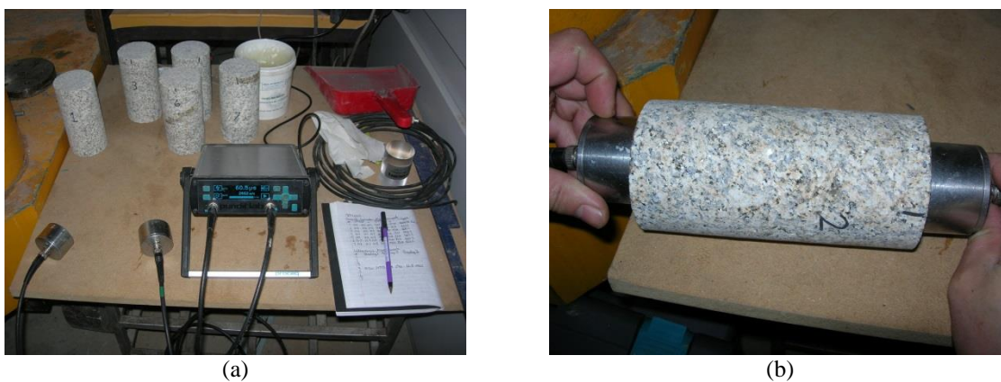
Figure 4-11. Ultrasonic pulse velocity testing of granite cylinders: (a) test equipment and set-up; and (b) performing a test on specimen RG2
