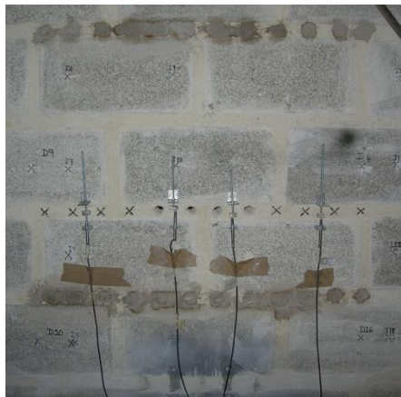
Figure 5-7 Photo of the drilling process during the single tube-jack test in the 4 th horizontal mortar joint
