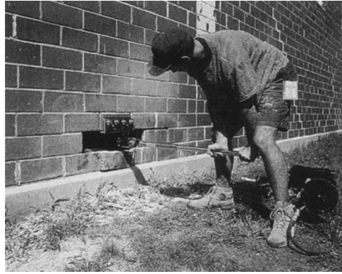
Figure 2-2 Bond wrench test being performed to determine the flexural bond strength [9]
