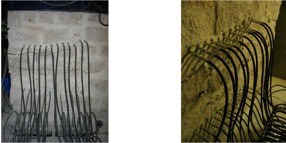
Figure 5-57 Complete double tube-jack test setup on the irregular wall
