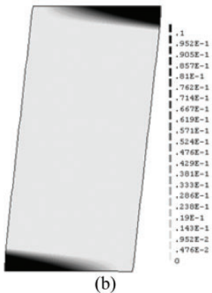
Figure 4. CS02 wall: (a) force-displacement curve; (b) maximum principal strains at the post peak.
