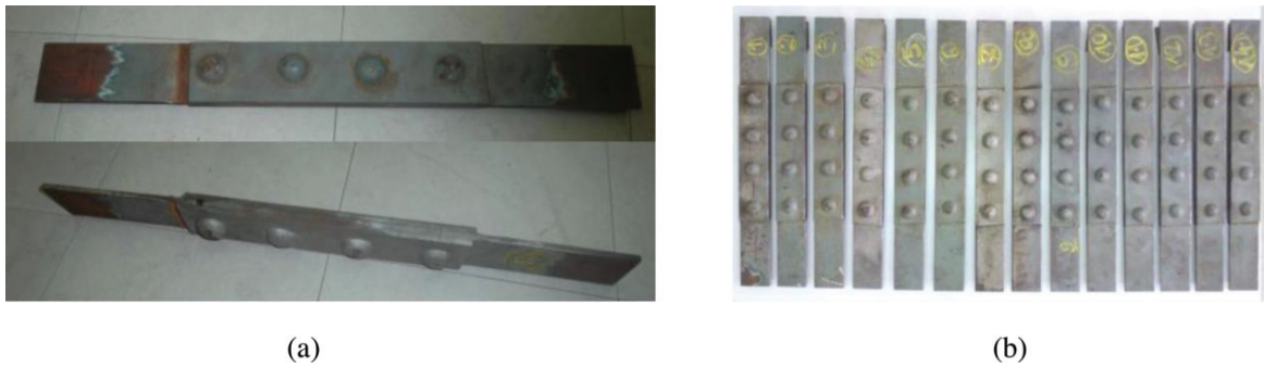
Fig. 5. Riveted specimens from the Eiffel Bridge (Portugal) (original joints sliced from girders web) [10-13].
