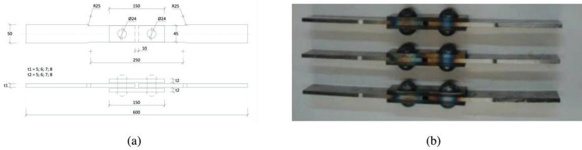
Fig. 4. Riveted specimens fabricated from puddled iron pieces from the Fão Bridge (Portugal) [10-13]; (a) layout of the specimens; (b) some examples of the fabricated specimens (plate surfaces were machined and holes drilled).
