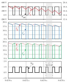
Fig. 6. Simulation results of the SSTL active rectifier in a detail of 600  $\mu$ s: Grid current ( $i_g$ ); Voltage produced by the SSTL active rectifier ( $v_{an}$ ); Current in the diode bridge ( $i_d$ ); Current in the bidirectional cell ( $i_b$ ); Control signal of the IGBT ( $v_s$ ).
