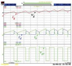
Fig. 10. Experimental results of the SSTL active rectifier: Power grid voltage  $(v_g: 50 \text{ V/div})$ ; grid current  $(i_g: 1 \text{ A/div})$ ; Current in the diode bridge  $(i_d: 1 \text{ A/div})$ ; Current in the bidirectional cell  $(i_b: 1 \text{ A/div})$ ; Gate-emitter voltage of the IGBT  $(v_{ge}: 15 \text{ V/div})$ .
