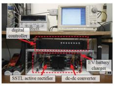
Fig. 8. Experimental setup of the EV battery charger where is incorporated the SSTL active rectifier combined with a dc-dc converter.
