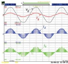
Fig. 9. Experimental results of the SSTL active rectifier: Power grid voltage  $(v_g: 50 \text{ V/div})$ ; grid current  $(i_g: 5 \text{ A/div})$ ; Current in the diode bridge  $(i_d: 2 \text{ A/div})$ ; Current in the bidirectional cell  $(i_b: 2 \text{ A/div})$ .
