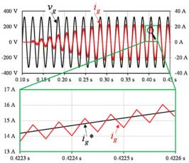
Fig. 3. Simulation results of the SSTL active rectifier during the initial phase of the EV battery charging process: Power grid voltage  $(v_g)$ ; Grid current  $(i_g)$ ; Grid current reference  $(i_g *)$ .
