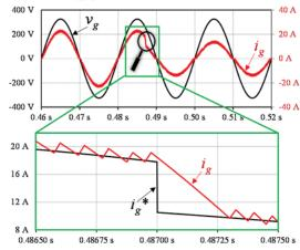
Fig. 4. Simulation results of the SSTL active rectifier during a transient variation in the power from 3.6 kW to 3 kW: Power grid voltage  $(v_g)$ ; Grid current  $(i_g)$ ; Grid current reference  $(i_g^*)$ .
