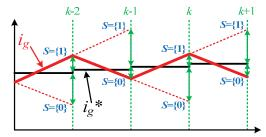
Fig. 5. Principle of operation of the SSTL active rectifier state selection
