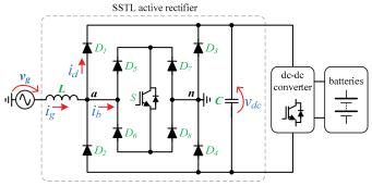
Fig. 1. Circuit topology of the single-switch three-level (SSTL) active rectifier for applications of battery chargers for electric vehicles (EVs).
