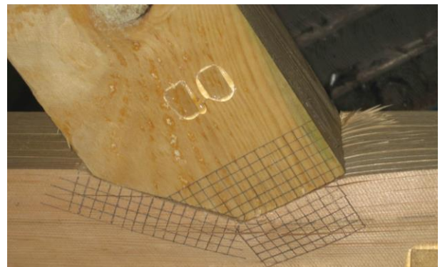
Figures 31 and 32 – Rafter force according to the displacement of the front-notch surface concerning all the 60°_tv25_200SL specimens (left). Crushing at the front-notch and at the rear of the bottom-notch surfaces (right).
