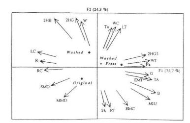
Figure 2. Vector map of changes of mechanical and thermal properties of cotton fabrics due to washing and pressing
