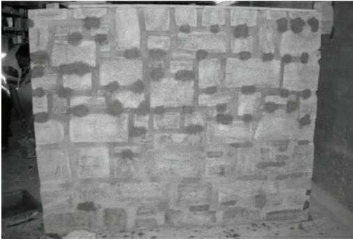
Figure 2. Construction of the semi-irregular masonry wall.
