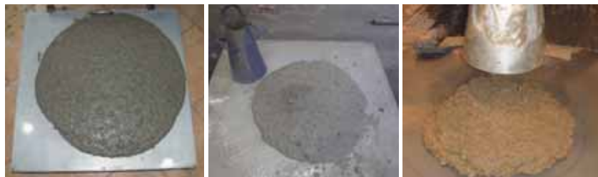
Figure 2. Different visual appearance of fresh concrete in different laboratories
