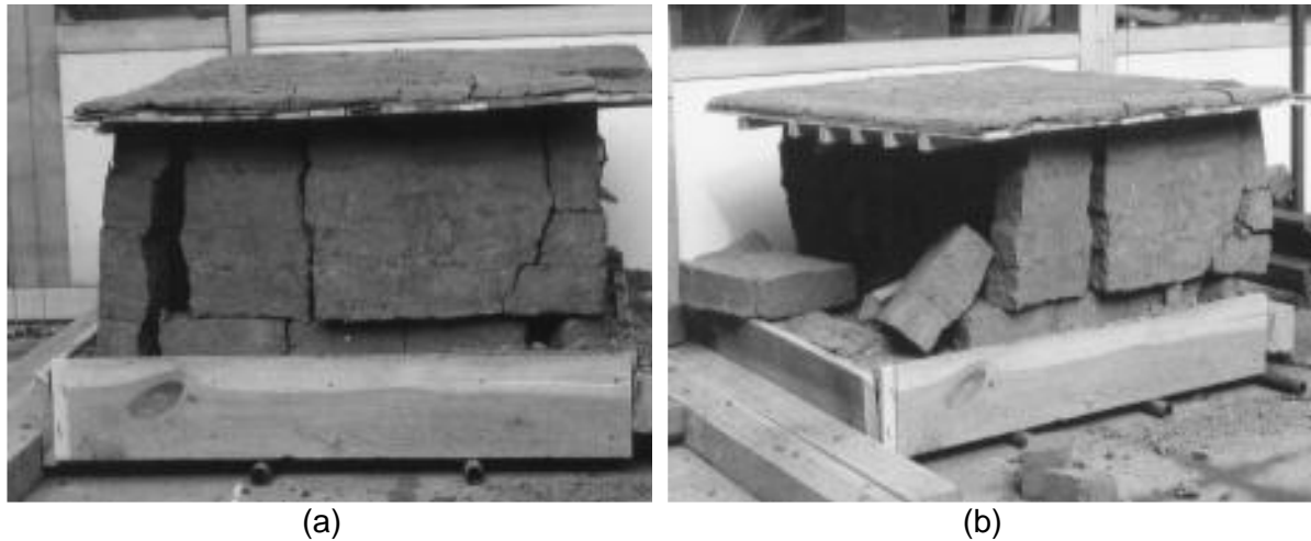
Figure 14: RE model with square plan developed a large crack after the 2 nd stroke, (a) one part separated after 3 rd strokes and (b) collapse after 4 th stroke ( Minke, 2001 )
