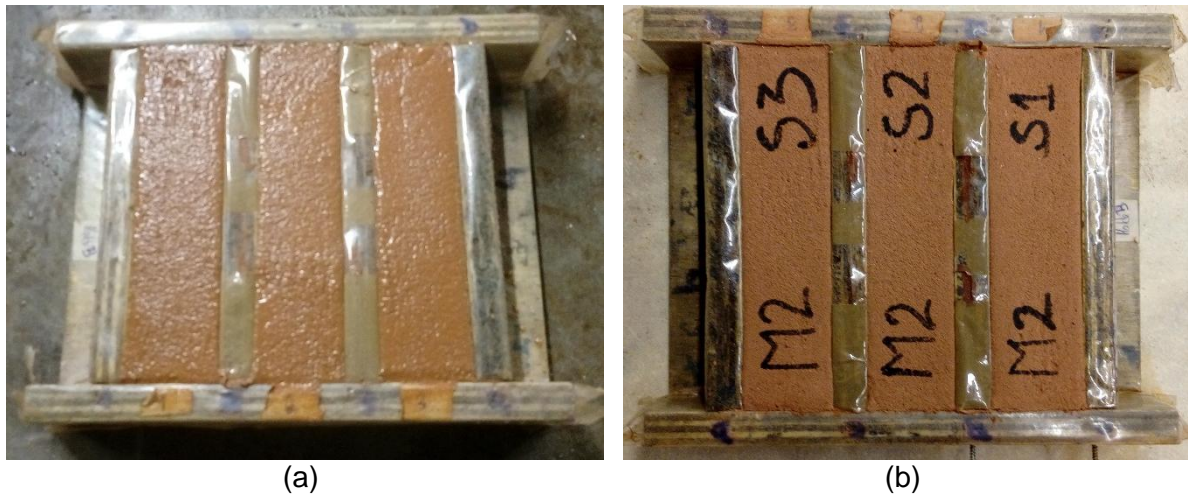
Figure 51: Earth mortar/M2 in (a) fresh state and (b) hardened state before demoulding
