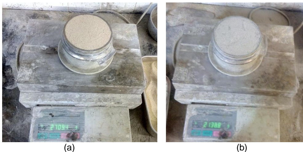
Figure 41: Mass of the material weighed in 1000ml container for (a) sand and (b) cement
