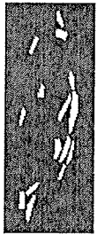
Figure 22. Image resulting from the application of the Particle Area Filter function to the image of Figure 21.
