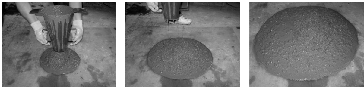
Fig. 3.12- HPFRC spread obtained on the slump flow test for mix B with 90 \text{ kg/m}^3 steel fiber.
