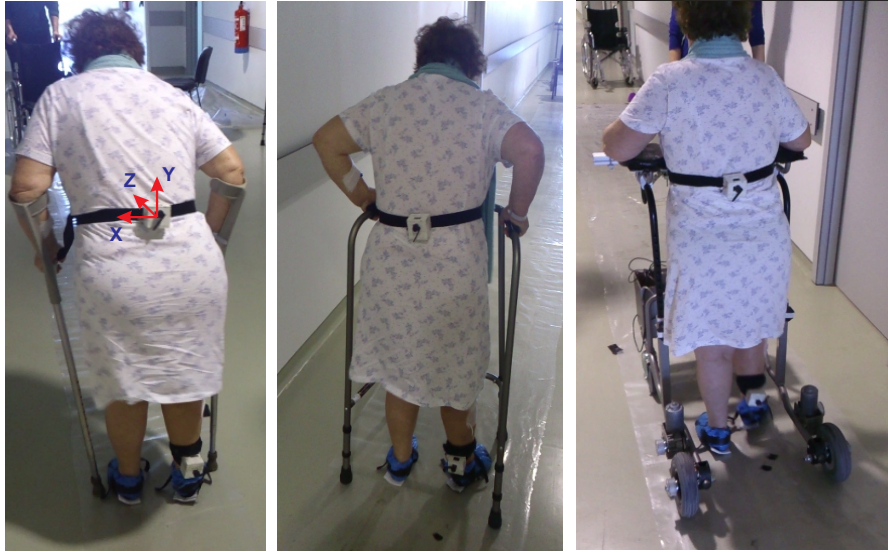
Figure 5.1: ADs used in this study. Left image: Crutches; center image: standard walker; and right image: RFS ASBGo walker. In the left image it is represented the axis of the sensor, used in all experiments.
