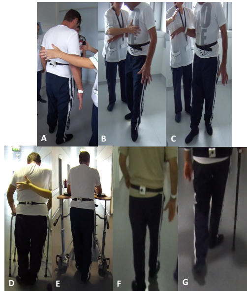
Figure 6.9: Postural stability evaluation tests with the patient of case 1: A- Comfortable stance (CS); B- Left semi-tandem stance (SSL); C- Right semi-tandem stance (SSR); D – Standard Walker; E- ASBGo walker; D- Without Assistance; and G – One Crutch.
