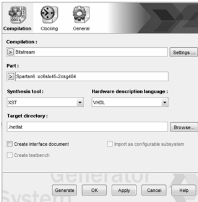
Figure 4-37: System generator compilation settings.
