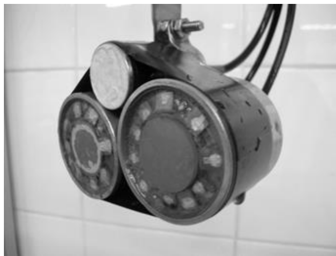
Figure 2-10: PVDF 4x28µm (Left), PZT 110µm (Top), PVDF 110µm (Right),
