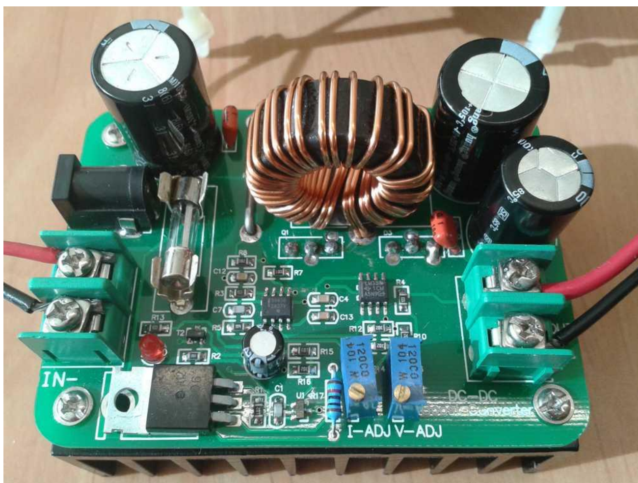
Figure 4-23: 600W 10-60 V to 12-80 V Boost Converter.
