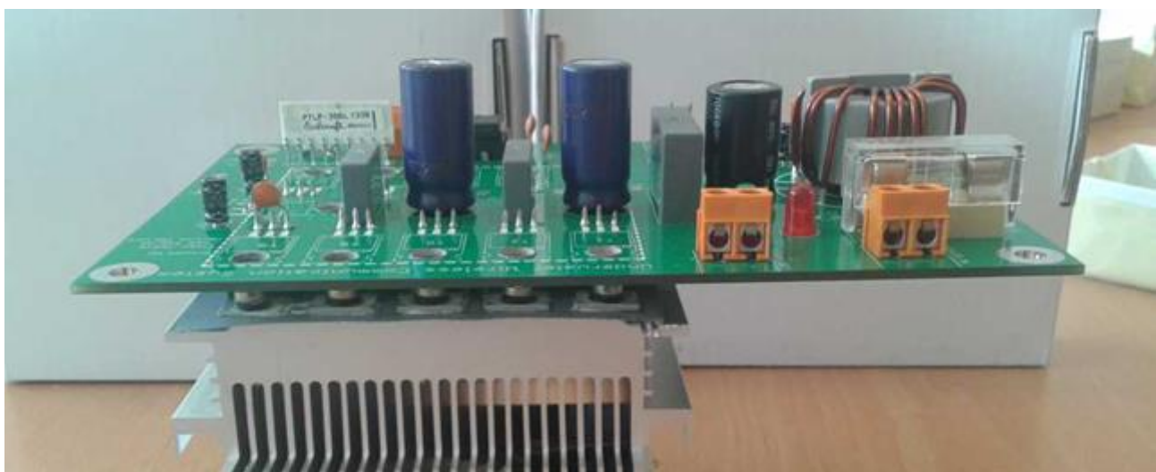
Figure 5-35: Cooler and fan setup.
