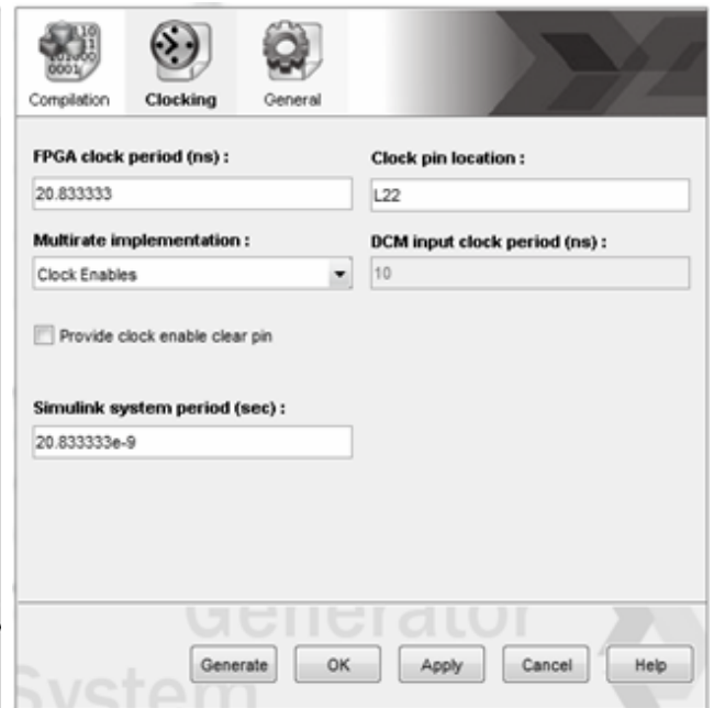
Figure 4-38: System generator clocking settings
