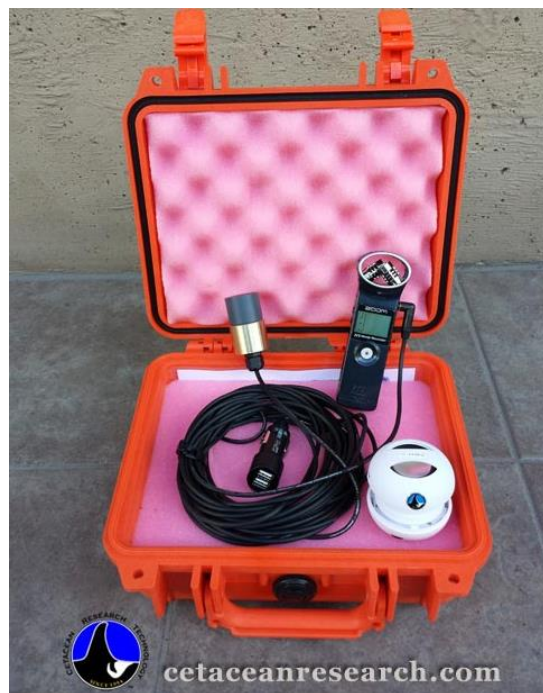
Figure 2-9: Underwater Recording Systems
