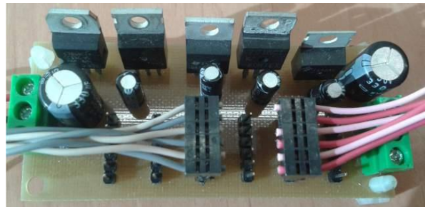
Figure 5-11: Voltage regulator prototype PCB.
