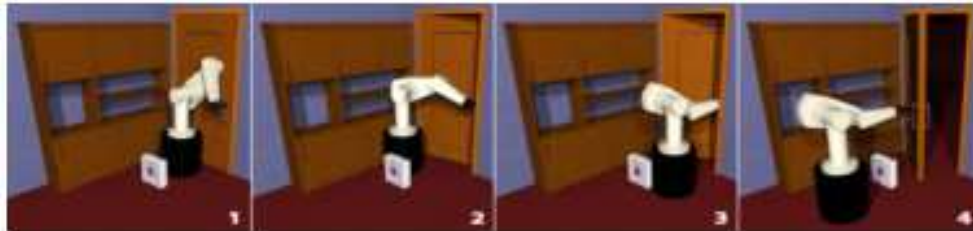
Figure 2.5: Simulation of the movement planning to open a door using Stilman's et al., RRT method. Note that the robot must avoid joint limits and the box placed in random positions to successfully complete the task (Stilman, 2010).
