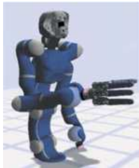
Figure 2.6: Simulation of the robot Rollin' Justin used to test human-like geometry planning (Zacharias et al., 2011).
