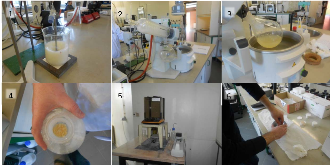
Figure 3.3 – Titanium dioxide preparation process – 1) Precipitation; 2) Rotary evaporation; 3) Sol in the rotary evaporator; 4) Dried gel; 5) Weighing of the gel in a balance; 6) Crushing in an agate mortar
