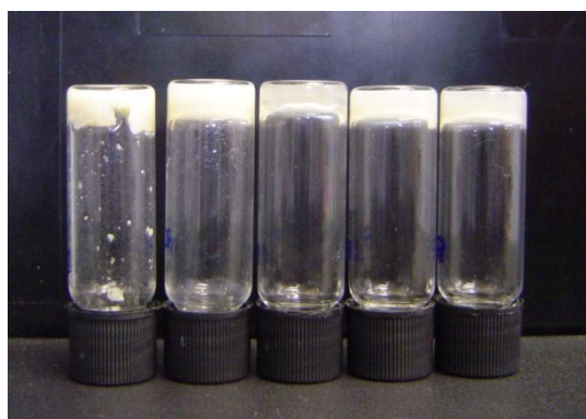
Figure S5. Gels obtained by addition of GdL to alkaline solutions of 7b ; Concentrations from left to right: 0.66, 0.60, 0.60, 0.49 and 0.41 wt%; pH from left to right: 3.82, 4.55, 5.81, 4.75 and 4.23.
