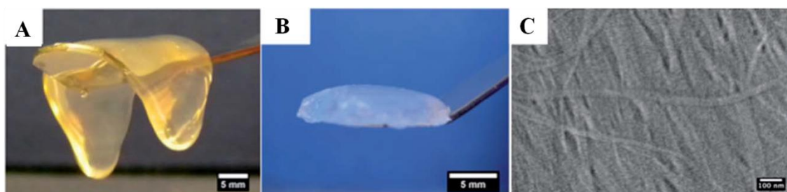
Figure 20. A) Photograph of the membrane formed by 6-Br-2-ONaph-Ala-Val triggered by \text{CO}_2 after 3 hours, held over a metal spatula; B) photograph of the membrane shown in A), 12 hours after addition of GdL to further lower the pH to approximately 4.0, held over a metal spatula; C) Scanning electron microscopy (SEM) image of air-dried membrane shown in A). For A) and B), the scale bar represents 5 mm; for C), the scale bar represents 100 nm (adapted from ref. 128 ).
