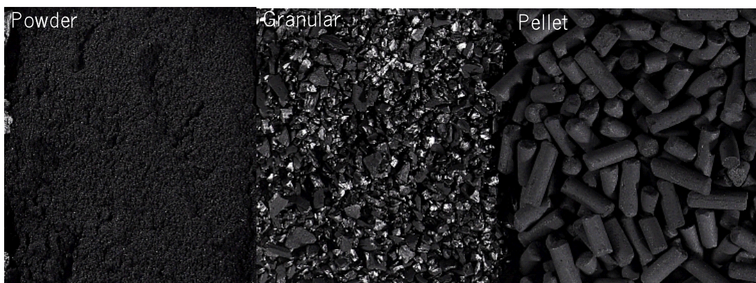
Figure 2.4. Different granulometries of AC. Pictures adapted from www.desotec.com (January, 2015).
