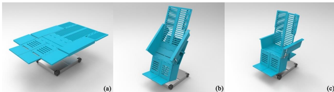
Figure 27 - “Transforming bed” concept ideas: a) Bed; b) Standing Frame; c) Wheel chair.
