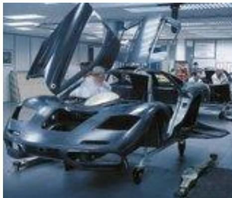
Figura 5 – Chassis monoque do McLaren F1 [16]
