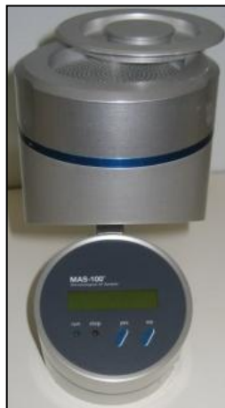
Figure 5 - Microbiological air impactor (Merck Air Sampler, MAS-100)
