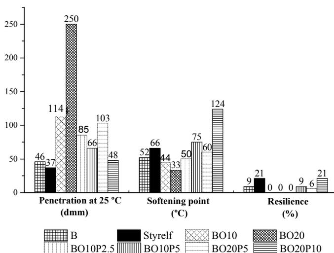
Fig. 2 – Penetration, softening point (R&B) and resilience test results of conventional bitumen and modified bitumens
