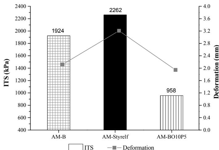
Fig. 5 - Indirect tensile strength and deformation at failure results of the studied asphalt mixtures
