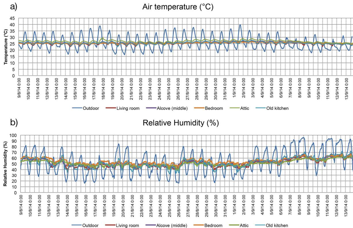
**Figure 12.** Case study 2 performance during summer season. (a) Indoor and outdoor air temperature profile; (b) Indoor and outdoor relative humidity profile.
