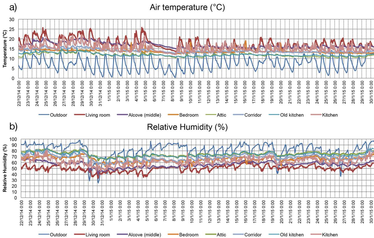
**Figure 14.** Case study 2 performance during winter season. (a) Indoor and outdoor air temperature profile; (b) Indoor and outdoor relative humidity profile.
