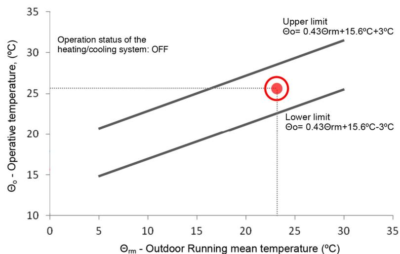
**Figure 13.** Thermal comfort temperature (operative temperature) in the living room during summer monitoring, based in the relation between the limits of the indoor operative temperature ( $\Theta_o$ ) for buildings without mechanical air-conditioning systems as a function of the exponentially-weighted running mean of the outdoor temperature ( $\Theta_m$ ) (adapted from [22]).
