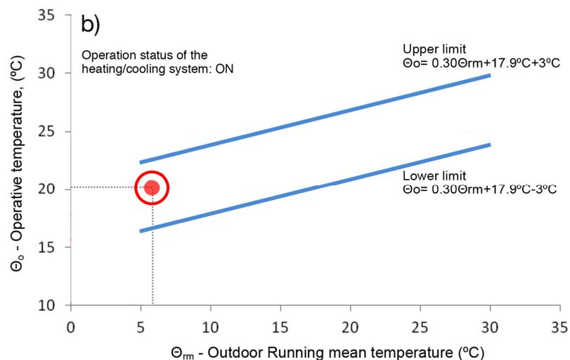
**Figure 15.** Thermal comfort temperature (operative temperature) in the living room during winter monitoring when the heating system was on, based in the relation between the limits of the indoor operative temperature ( $\Theta_o$ ) as a function of the exponentially-weighted running mean of the outdoor temperature ( $\Theta_{rm}$ ) (adapted from [22]).
