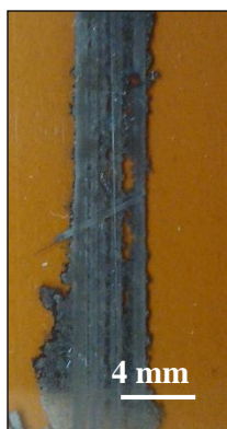
Figure 6.5 - Example of flooding of one layer of the printed silver-based ink (with drop spacing of 28.22 \mu\text{m} (900 DPI)) on a clean PI substrate.
