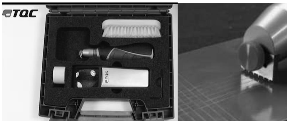
Figure 3.18 - The TQC Cross Cut Adhesion Test KIT (CC2000) at the left and Cutting tool accessory at right.
