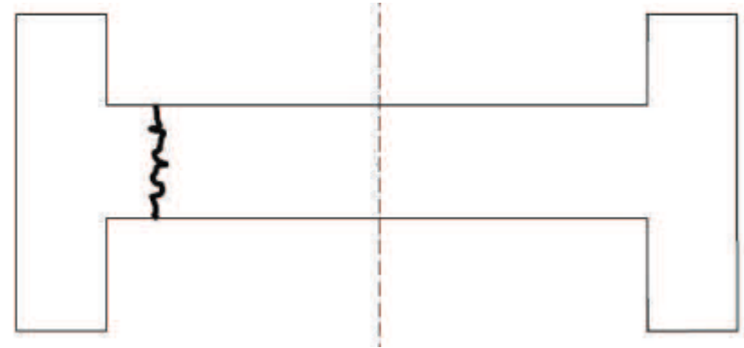
2nd crack: \approx 170 h (7 d) after casting
