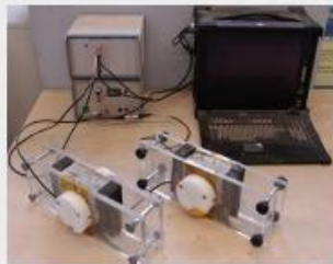
FreshCon setup for the simultaneous measurement of P-wave and S-wave transmission
