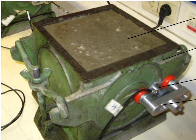
Fresh concrete Metal mold AE sensor Magnetic clamp
