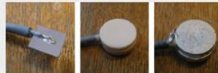
Smart Aggregates : embedded piezoelectric transducers (P-wave) left : piezoelectric patch; center : waterproof coating; right : smart aggregate
