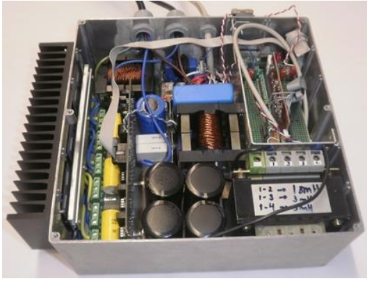
Fig. 3 Developed batteries charging system.
