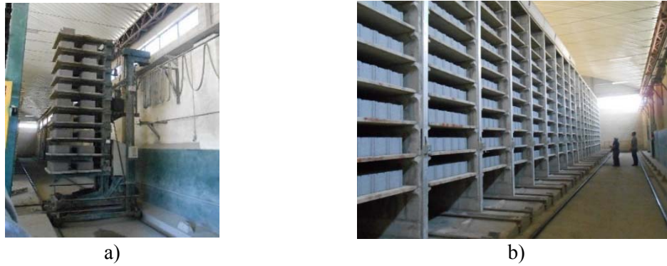
Figure 3: Manufacturing of CMU-PCC – Curing/drying: a) automatic transportation and b) curing chamber
