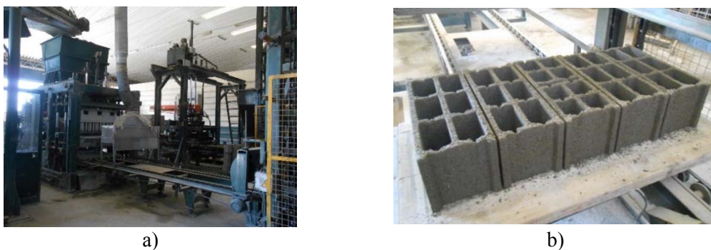
Figure 2: Manufacturing of CMU-PCC – Moulding: a) Moulding process and b) manufactured units
