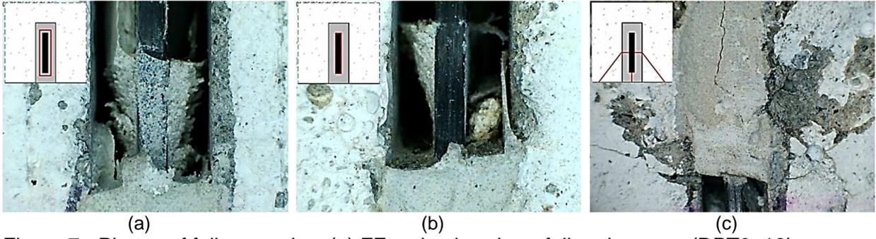
2 Figure 7 - Photos of failure modes: (a) FE: cohesive shear failure in epoxy (DPT3\_12h –
