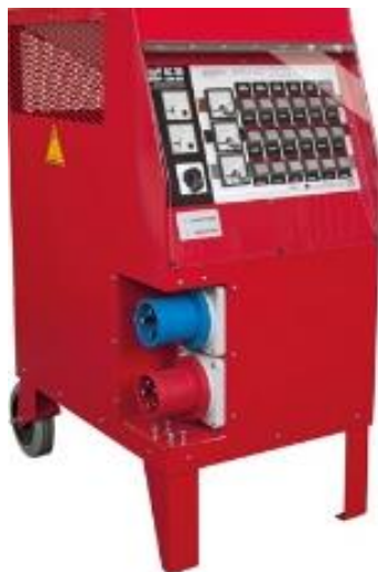
Figure 4.19 – Front view of the 30 kVA load.
