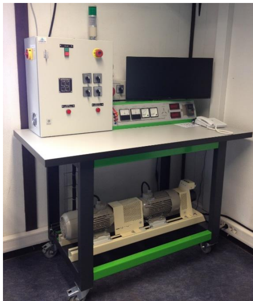
Figure 4.23 – EOLYP 1.2 kW wind turbine emulator.
