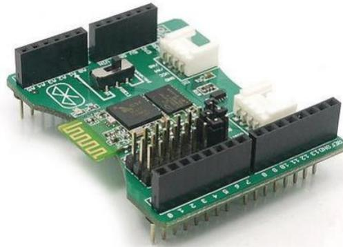
Figura 11 - Bluetooth Shield (Master/Slave)
