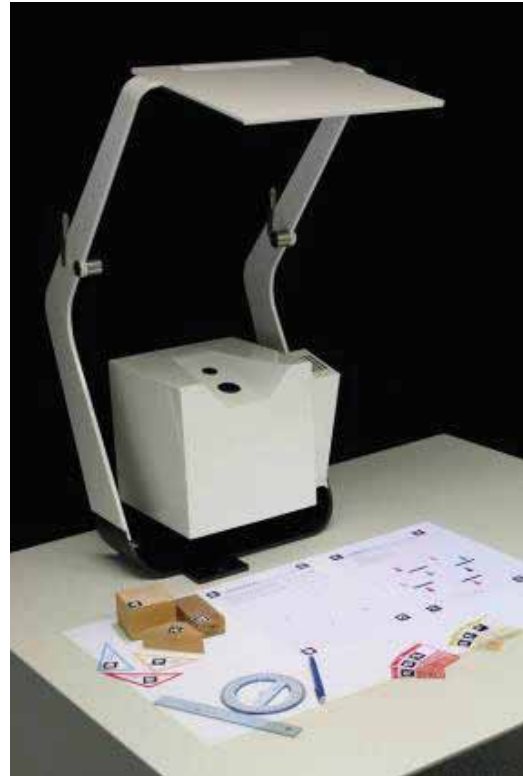
Figure 1. Our camera-projector on a table, along with various types of objects which can be augmented: sheets, cards, tools, and wooden blocks
