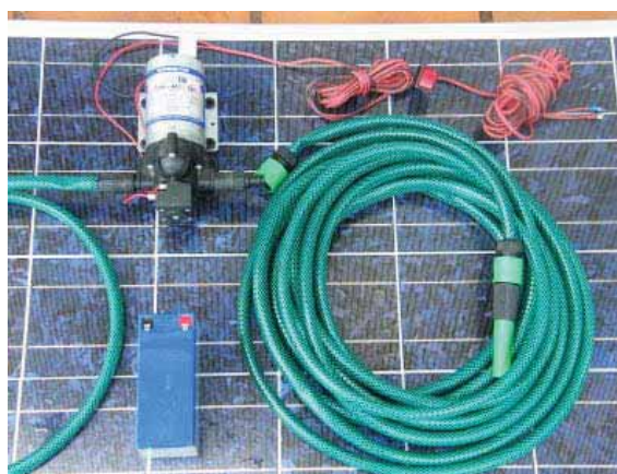
Figure 4. The solar pumping set
