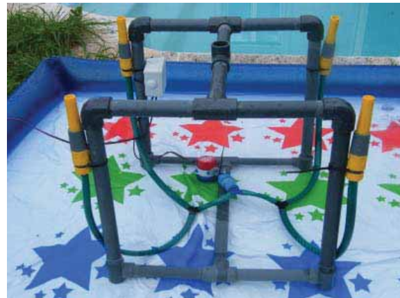
Figure 6. Structure with pump and hoses
