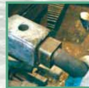
Upset socket depth and hole location gauge for accurate attaching
