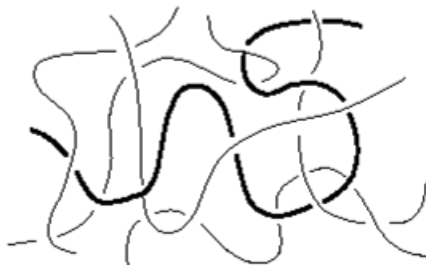
Figure 4 : Linear Polymer with Entanglements, adapted from (W.J. Briels 1998)
