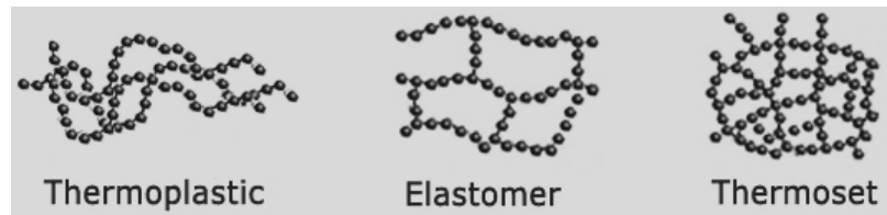
Figure 6 : Different types of Polymers, where, a small bead represents the monomer unit. Adapted from (Adhesivesandglues.com 2012)
